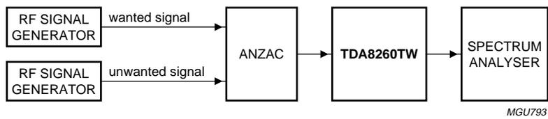
Fig.8 Test set-up.
