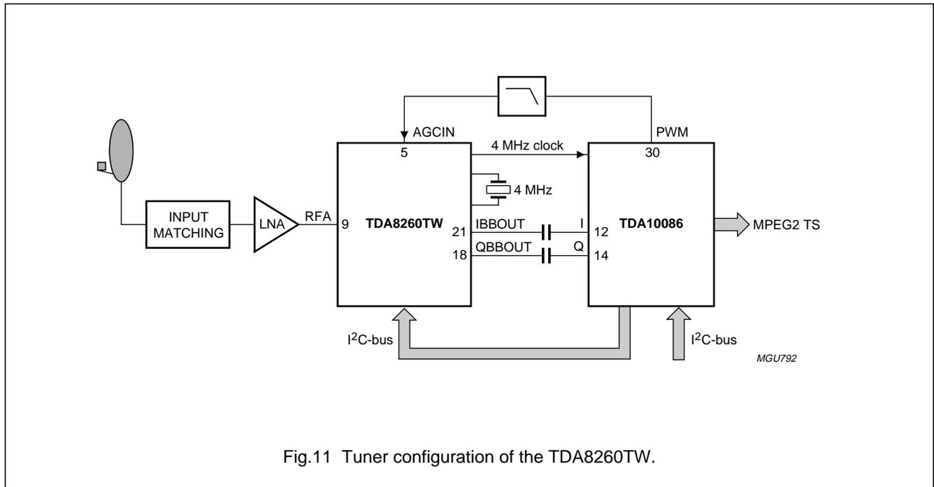
Fig.11 Tuner configuration of the TDA8260TW.
