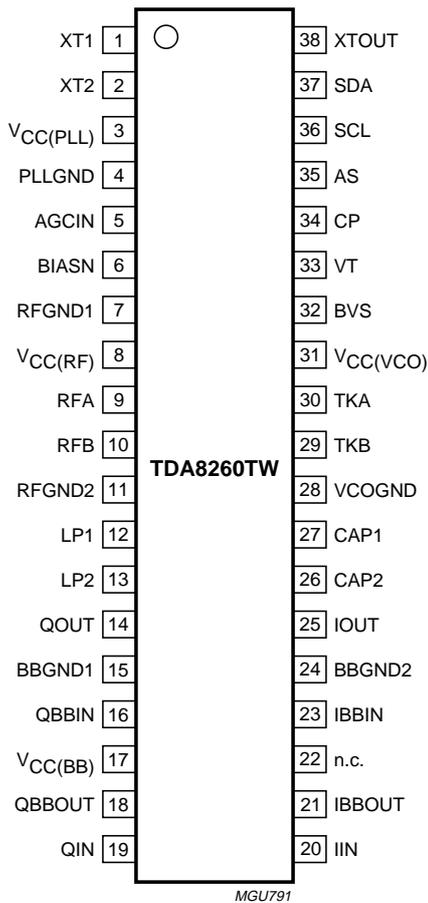
Fig.2 Pin configuration.
