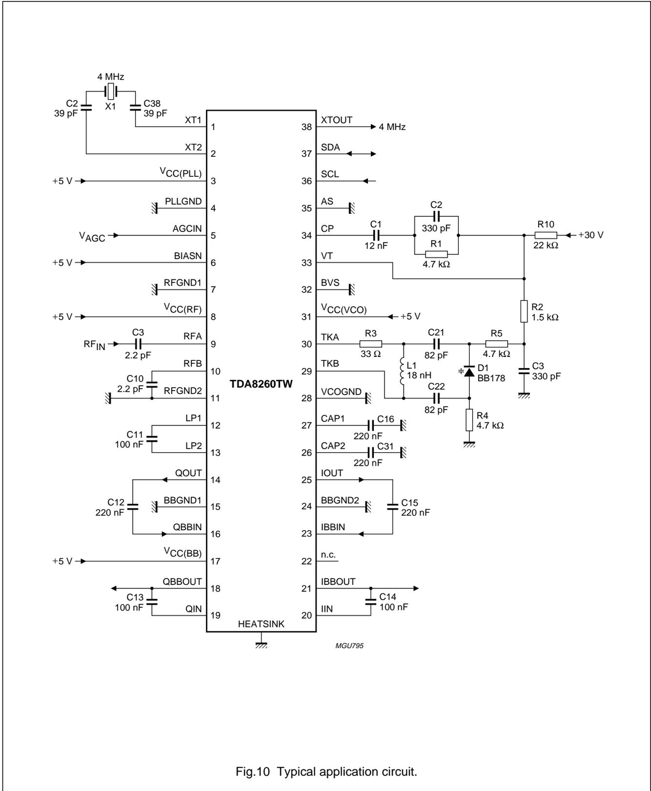
Fig.10 Typical application circuit.
